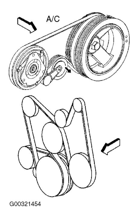
Fig. 1: Serpentine Belt Routing Courtesy of GENERAL MOTORS CORP.
